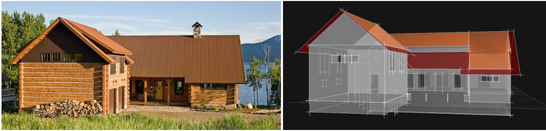
Figure 2a (Left) Subject Case: A Residence on Henry’s Lake, Idaho; (Author Name) Design 2007. Image credit: J. K. Lawrence. Figure 2b (Right) Thermal model generated using AutoDesk Ecotect Analysis 2010. Image Credit: Evan Possley.
